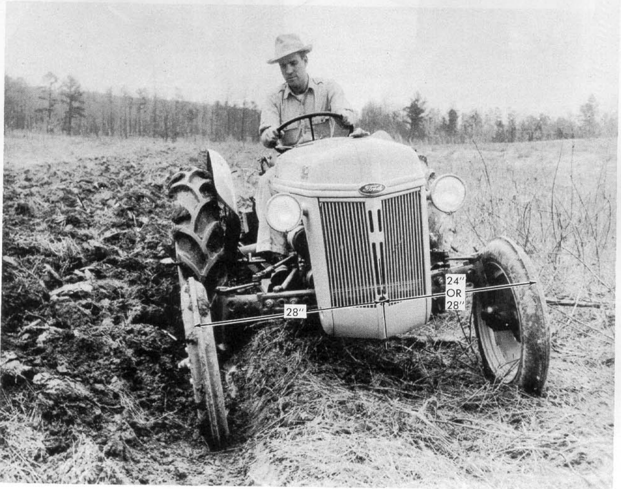
Figure 8 Recommended Front Wheel Setting
